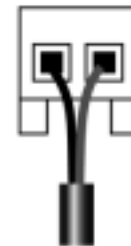
J3 Connector Flow Switch (Cable Side) Shown while Plugged into Circuit Board
